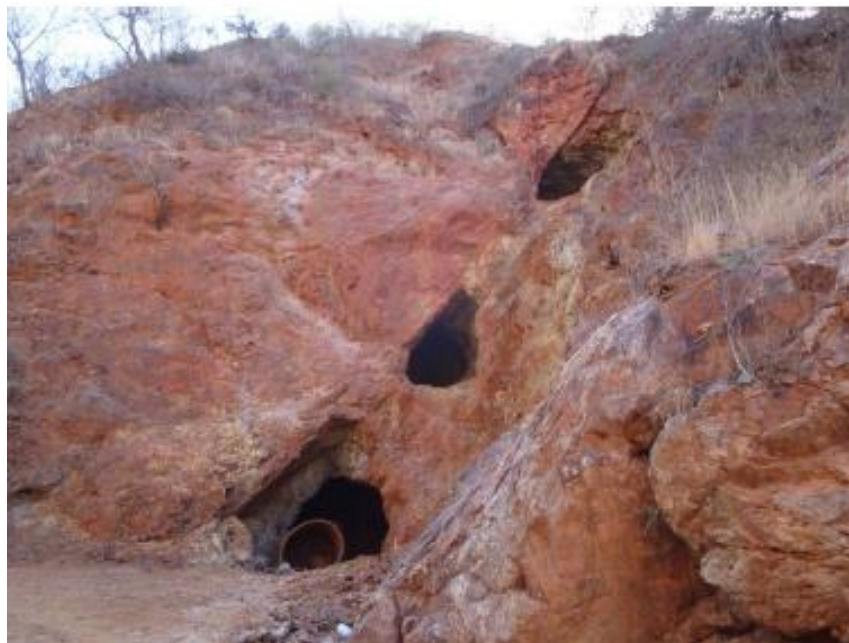
Fig. 3.3 Photograph of the Tres Amigos mine showing how the vein thickness, as indicated by the size of the workings, decreases up-dip. This is caused by the vein terminating against a 060^\circ striking, sub-vertical, oblique, strike-slip. All the veins in the San Jose de Gracia area terminate in this manner and this is the main reason why they are difficult to identify in surface outcrop. 213657 E 2898043 N, looking towards 066^\circ .
