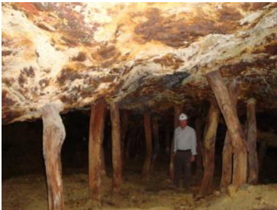
Fig. 3.5 18^{\circ} to 050^{\circ} dipping stope over 2 m high within the La Prieta mineralized area. Meta-sediments form the footwall and hangingwall of the stope. Photograph looks towards 090^{\circ} .
